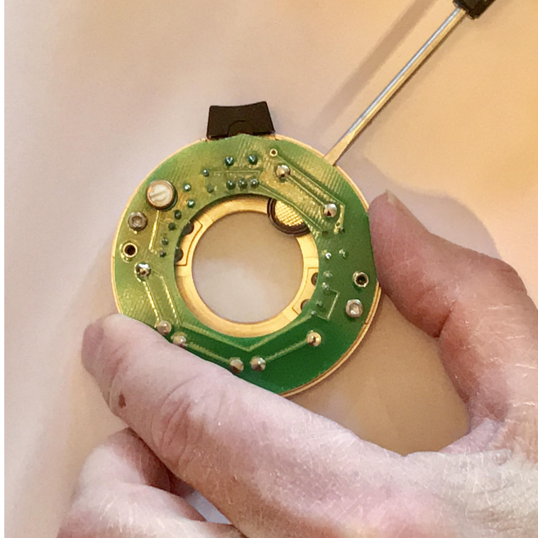
Figure 6 - How to push an SR44 battery out of its Photo-Bluminator II battery holder.
