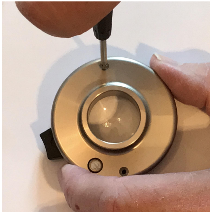
Figure 3 -Unscrewing the screws on the back case of the Photo-Bluminator II with the phillips head screwdriver.
